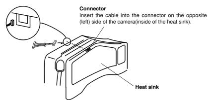
Remove the blank panel (right side of camera), then feed the cable (supplied with the board) through the rectangular opening under the top panel and insert it into the connector on the opposite side.
